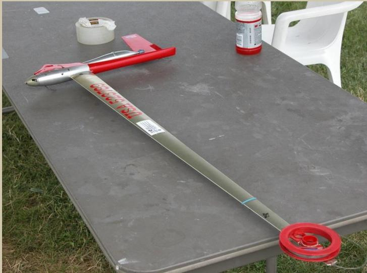
A typical FAI 0.15 cubic inches (2.5cm<sup>3</sup>) speed model – with control lines stored on reel between flights. Very long inboard wing acts as a fairing for the control lines, greatly reducing aerodynamic drag
